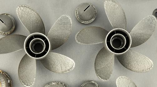
The processing speed is 5-20 cm<sup>3</sup>/h depending on the space utilization. The generated parts have a homogeneous structure and a density of almost 100 %. Not only the physical but also the mechanical properties of the produced components comply with cast structures. The laser of the selective laser melting machine which is placed at the Fraunhofer IPK has a power of 400 W.
