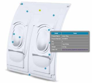
Digital visualization of an aircraft interior wall
