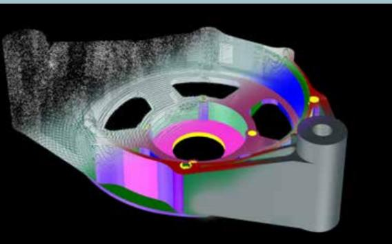
Classically, data points – sometimes up to several million of them – are pre-processed before model reconstruction can begin at all. Incorrectly detected points are discarded, the entire point cloud is divided up into subsections, and the point density is reduced.
