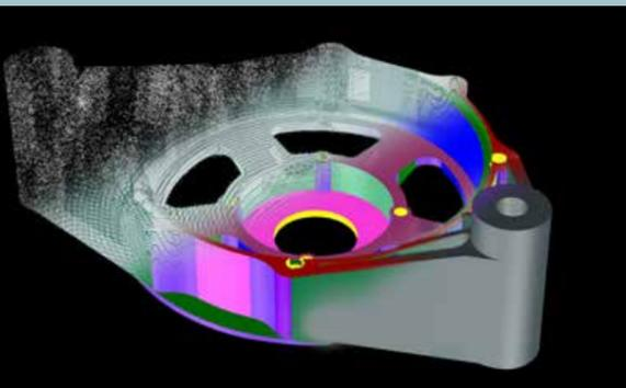
Classically, data points – sometimes up to several million of them – are pre-processed before model reconstruction can begin at all. Incorrectly detected points are discarded, the entire point cloud is divided up into subsections, and the point density is reduced.
