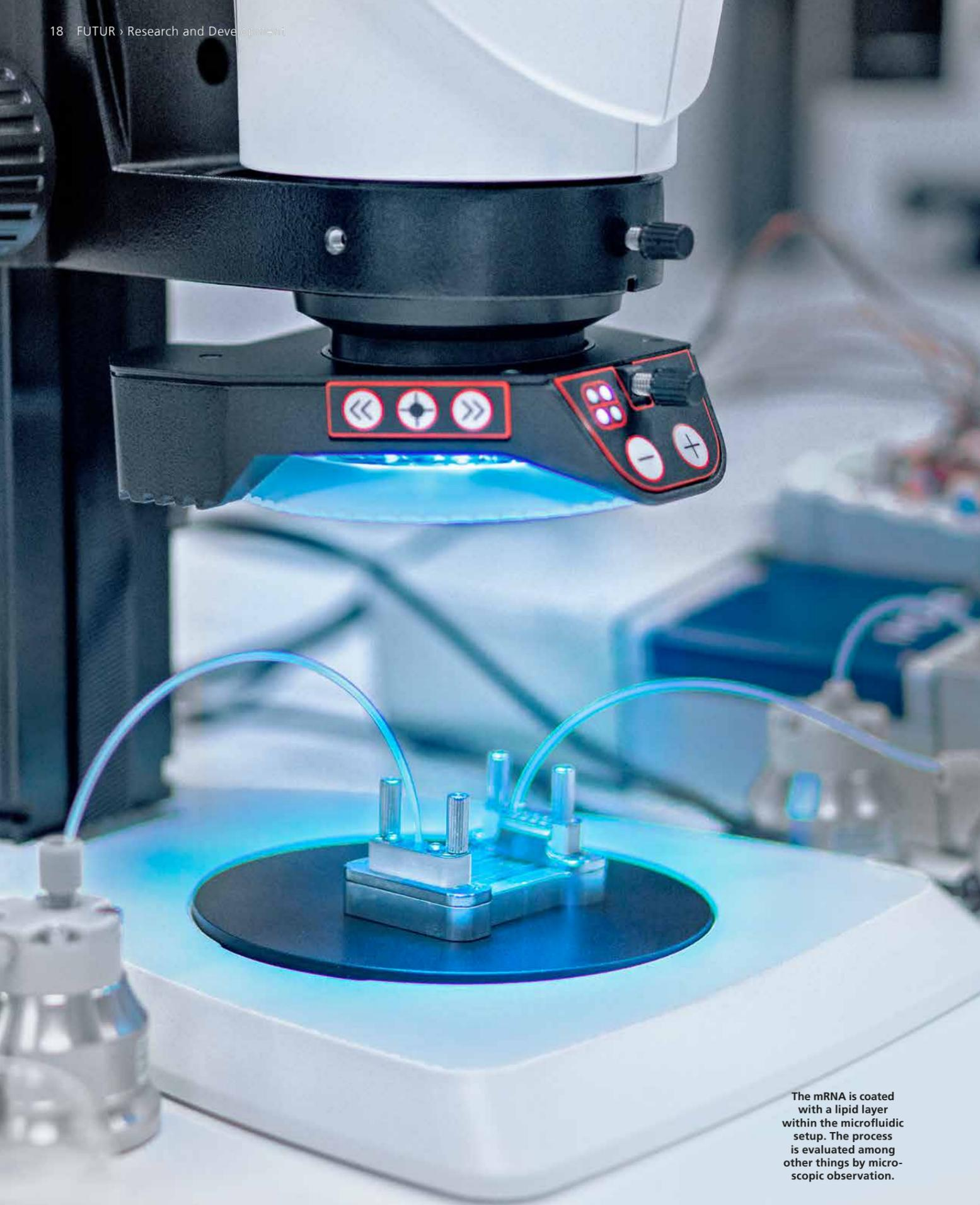
The mRNA is coated with a lipid layer within the microfluidic setup. The process is evaluated among other things by microscopic observation.
