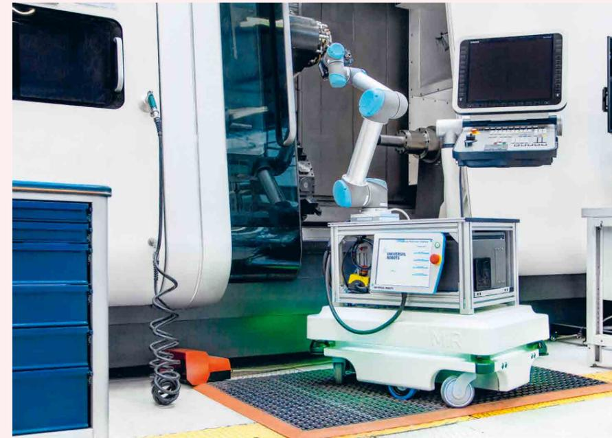
**The Tend-O-Bot demonstrator can load machine tools fully automatically. What requirements do you have in your company for a mobile helper such as this one?**
