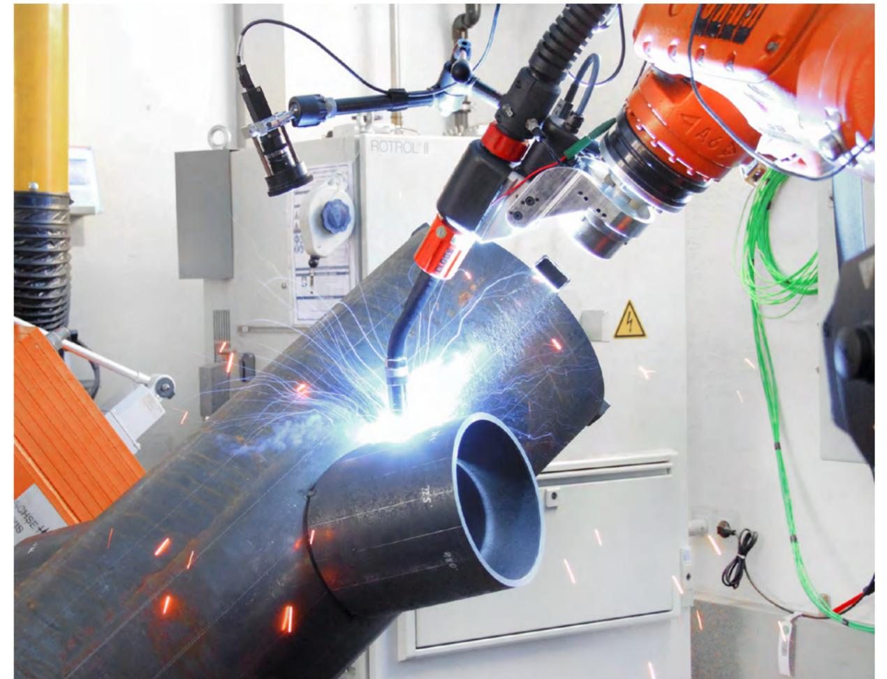
Gas shielded metal arc welding (GMAW) is used for the automated welding of pipe nodes. Tube nodes are an important structural element in steel construction, for example for the foundation structures of offshore wind turbines. © BAM
