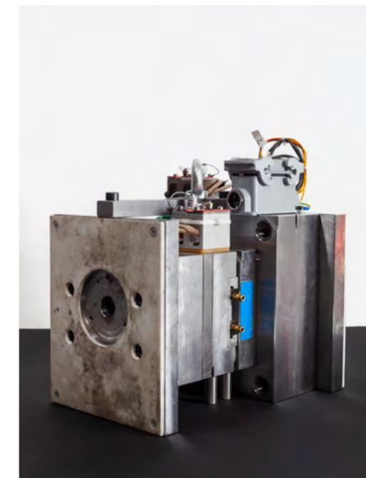
The Fraunhofer IPK team developed this injection molding tool for replicating the model components.
