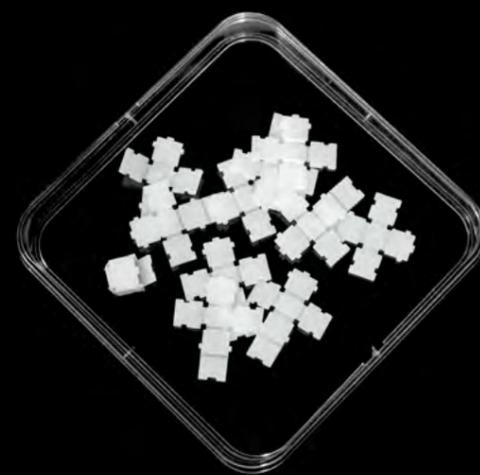
PHB as an energy reservoir in the cell. Once the plastic has been dissolved from the cell, it is still not ready for industrial use, because the hardening process takes far too long. The raw material has to be mixed with chemical additives in special post-production stages. The outcome is a plastic exhibiting similar characteristics to those of polypropylene (PP). Yet unlike PP, this plastic is completely biodegradable within a period of six to twelve months.
