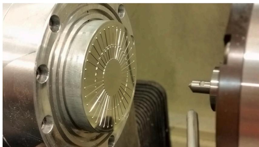
*Manufacture of a molding tool for the production of blood plasma separators based on micro-fluid principles with a minimal structural dimension of 15 µm*
