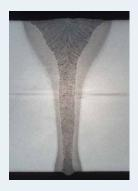
Narrow-gap submerged arc welding (above) on a 30 mm sheet costs 3,40 €/m, laser hybrid welding (below) only 0,48 €/m.
