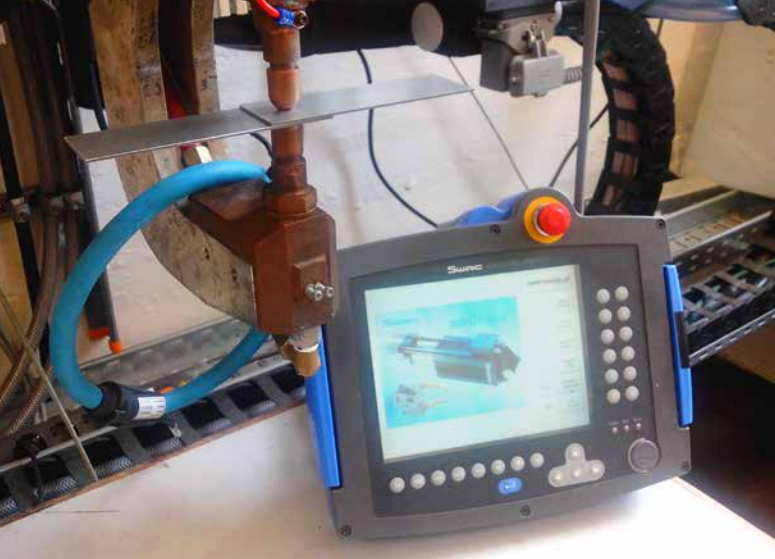
Welding gun for resistance spot welding
