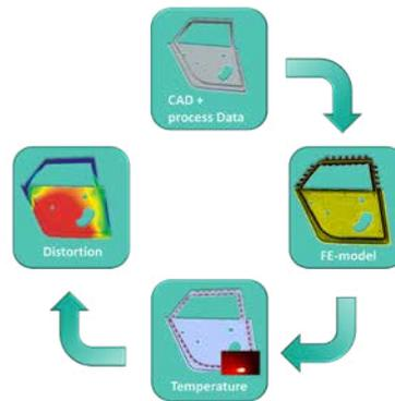
*Results of a welding simulation / Overview of process steps using the example of a car door*
