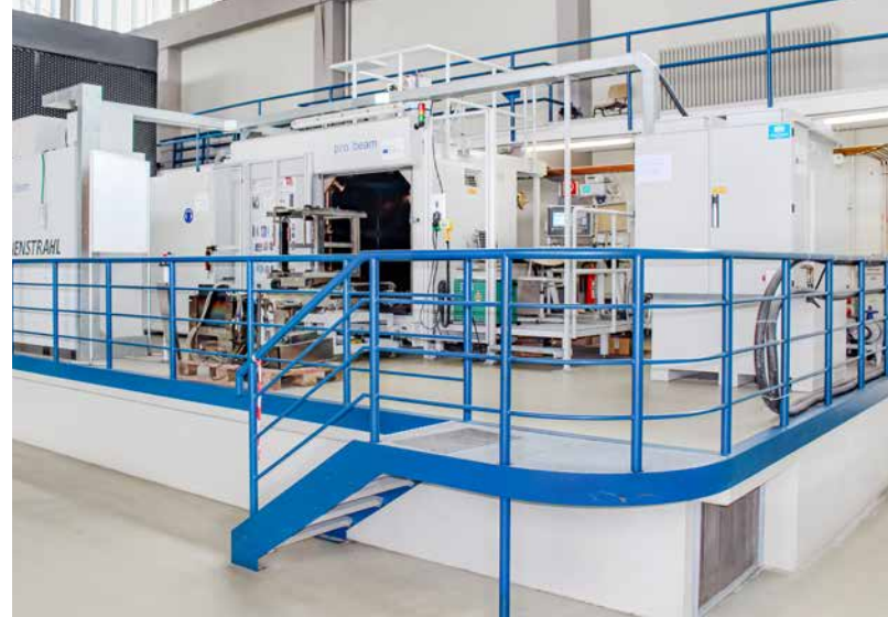
Electron beam system at Fraunhofer IPK ready for Wire Electron Beam Additive Manufacturing
