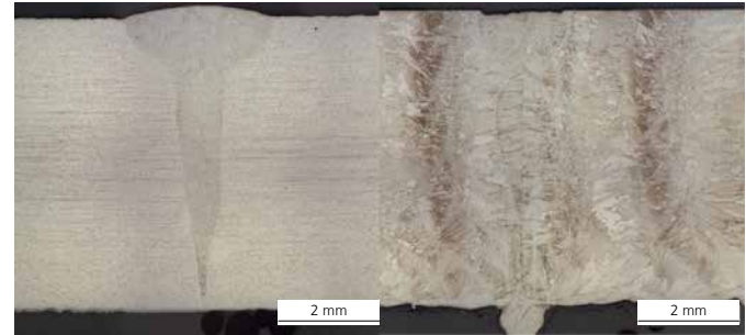
Left: Blind seam in a conventional material Right: Blind seam in an additive part
